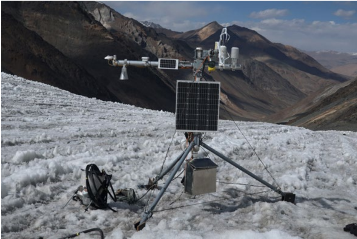
Figure 27. Automatic weather station on Zulmart glacier, installed in 2022.
