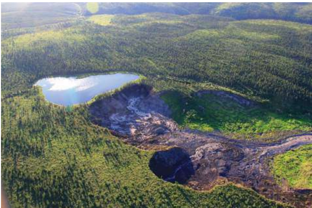
Abrupt permafrost thaw on the Peel Plateau in Canada. Thawing of ice-rich permafrost can cause abrupt ground collapse, which can further accelerate thaw and increase permafrost carbon emissions. For scale, the lake length parallel to the headwall of the thaw feature is 150m. CREDIT: SCOTT ZOLKOS
