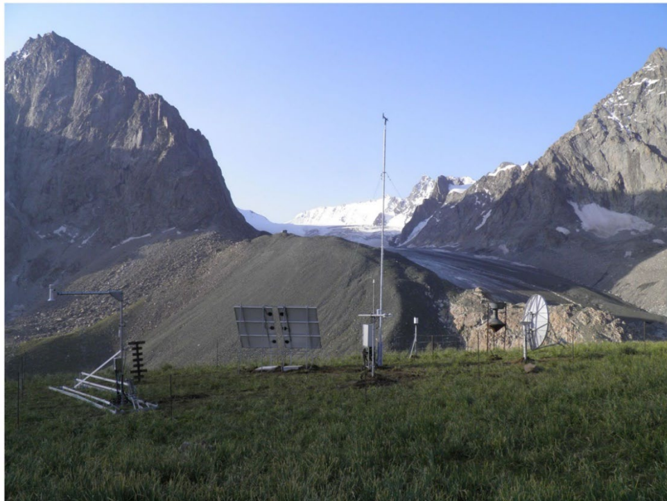
Figure 25. High-mountain hydrometeorological station near Golubin Glacier, Kyrgyzstan (CAWa)
