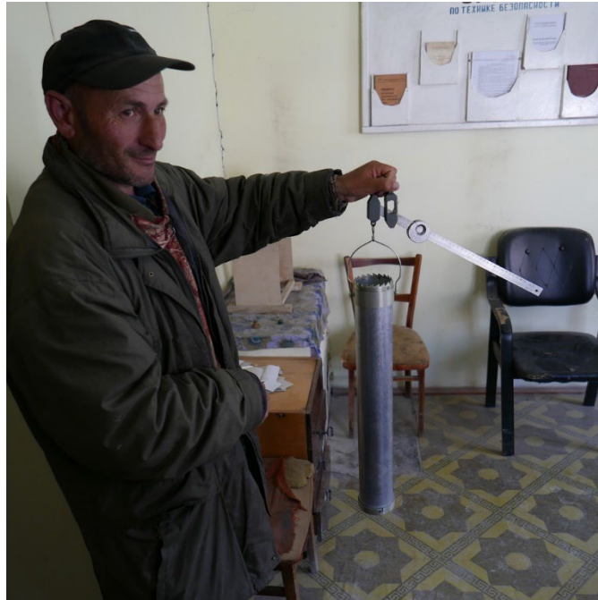
Figure 9. Manual snow measurements of snow height and water equivalent are made at many SYNOP stations in the region, but this data is not transmitted in real time via the WMO Information System (WIS). Soviet era equipment and protocols are still used, as seen here with the snow water equivalent sampler (Tajik Hydromet Station Iskanderkul).
