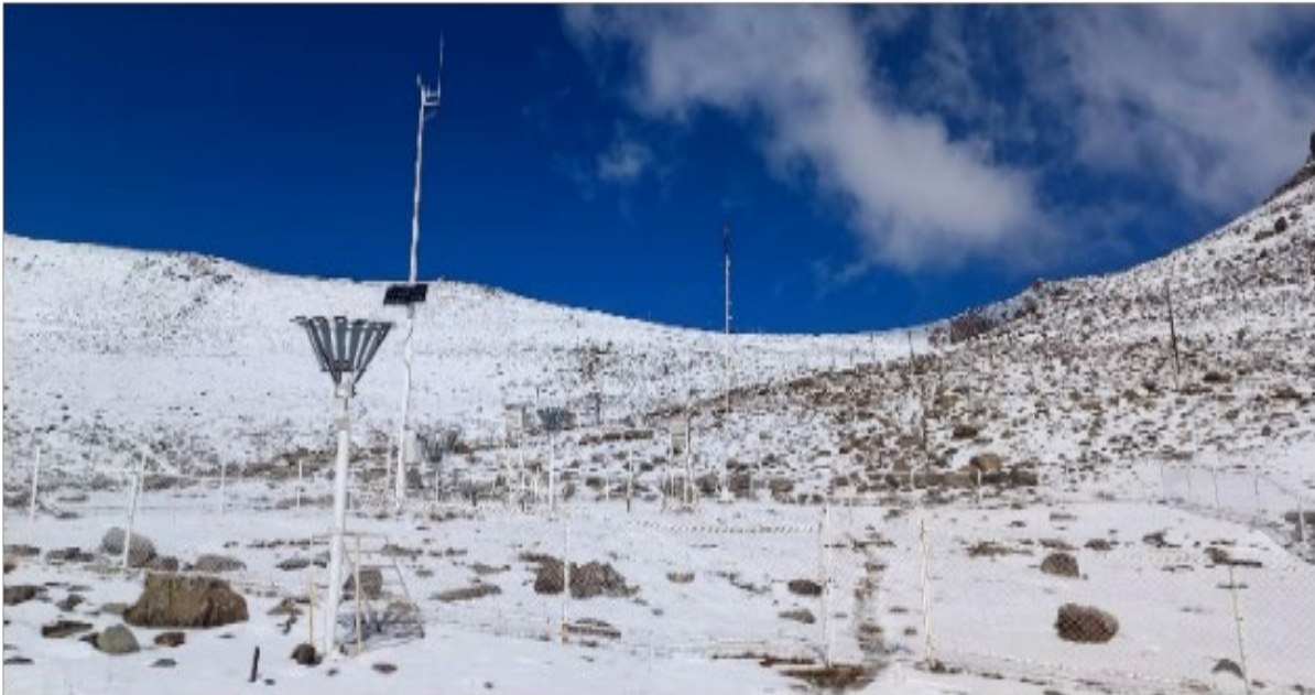
Figure 8. Snow observation station Too-Ashuu in Kyrgyzstan equipped with an automatic measurement station from the World Bank financed CAHMP project (S. Belekov).
